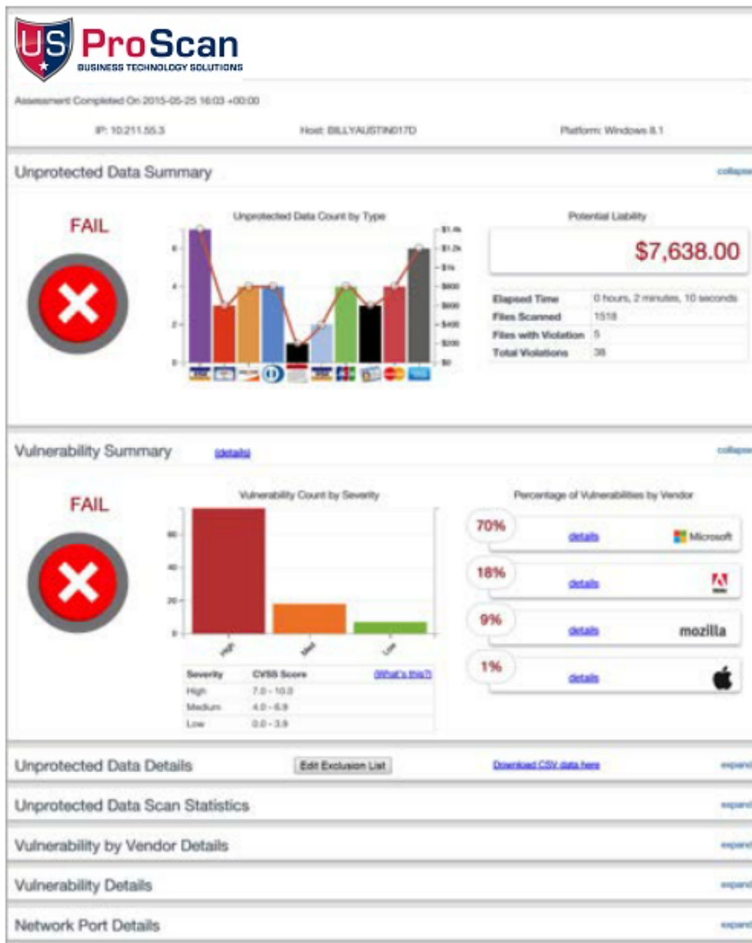
Figure 2: Sample Device Risk Report that includes data at risk, access information, vulnerabilities and the Security Number, the risk liability calculated in dollars.
